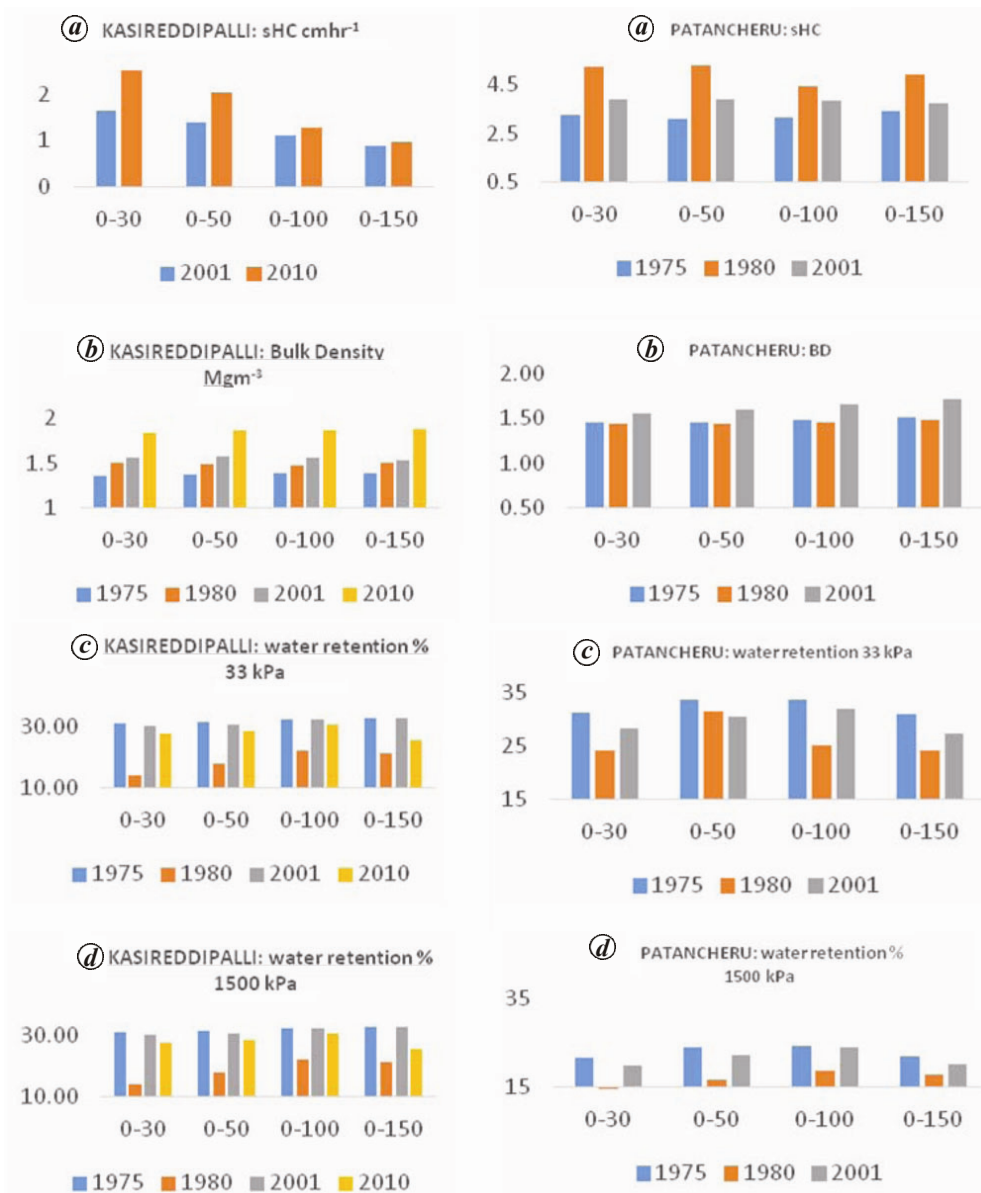
Figure 8. Changes in physical properties over time in black (Kasireddipalli) and red (Patancheru) soils: a , saturated hydraulic conductivity; b , bulk density; c , water retention (%) at 33 kPa; d , water retention (%) at 1500 kPa.
